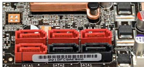
Traditional SATA connects interfere with bigger graphics cards and cause clutter
